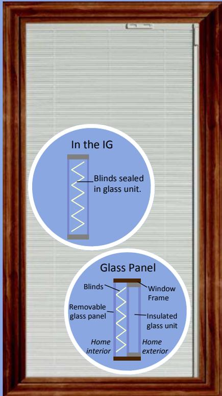
Lindsay's casement, awning and picture windows are available with mini-blinds. These blinds can either be contained in the IG Unit (the blinds are in the sealed glass), or contained by a separate removable panel of clear glass. Blinds contained in the IG Unit are available with optional argon gas but Soft Coat Low E is not available. Blinds contained by the separate removable panel of clear glass have all of the regular glass options available to these windows.
