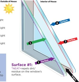
◆ Optimal energy retention is achieved with the lowest number. This measures inside temperatures from escaping to the outside.
